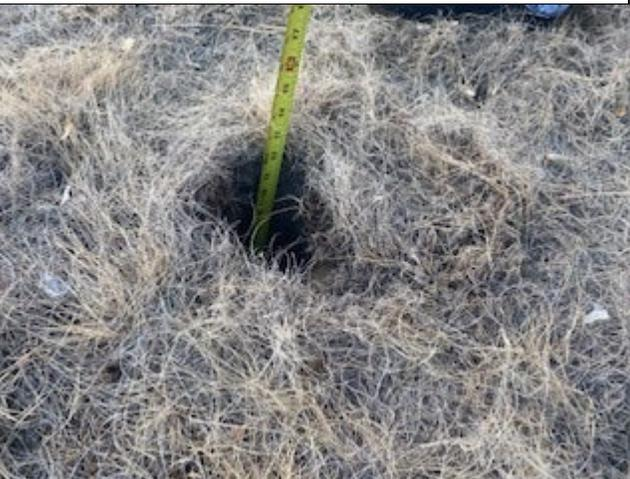
Typical depth verification and boring hole
