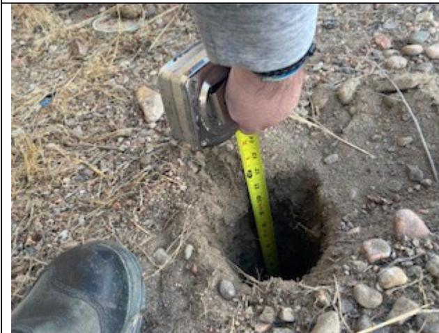
Typical depth verification and boring hole
